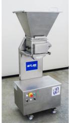
The granulating machine (GTS) has been designed for granulate solid food products continuously. The product is introduced into the hopper and then carried to special rotary blades, that process the product in granules. The granulating machine has a loading platform, where you can place the baskets for collection; alternatively, the handles are suitable for the anchoring of bags.
